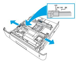
**3.** Adjust the paper-length guide by squeezing the adjustment latch and sliding the guides to the size of the paper being used.
