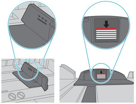
Figure 9-3 Tab for the paper stack
