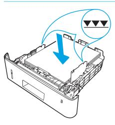
5. Slide the tray completely into the printer.
