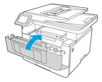
8. If no paper was jammed inside the print cartridge door, press the front door release button.
