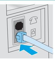
4. Connect the answering machine telephone cable to the telephone line out port on the rear of the printer.
