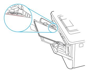
6. Press down on the tab on the right paper guide, and then adjust the paper guides so that they lightly touch the paper stack but do not bend the paper.
