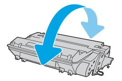
7. Align the toner cartridge with the tracks inside the printer, and install the toner cartridge until it is firmly seated.
