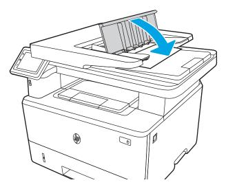
7. Open the scanner lid. If paper is jammed in the scanner lid, gently pull it out, and then close the scanner lid.
