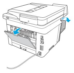
10. If jammed paper is visible, remove any jammed paper from the rear door area.
